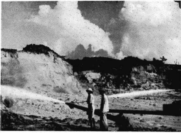
Counterbalanced monitors stripping overburden in an open-pit mine. Loosened overburden is often made to flow in the empty part of the pit; otherwise, it may be pumped behind the dikes that close off the pit.
