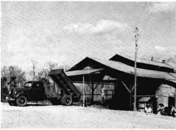
Unloading semiconcentrates at a small concentrator where the material is jigged, tabled, and, if necessary, further cleaned by magnetic separators to remove the associated minerals ilmenite, monazite, and magnetite.
